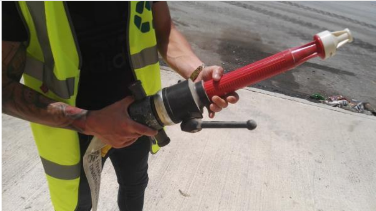
STEP 3: Attach the firefighting nozzle to the fire hose.
